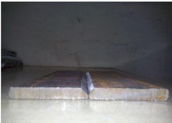
**Fig5: Single V Butt Joint before welding**
