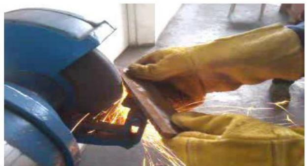
Fig-3: Edge Preparation (Single V butt Joint)
