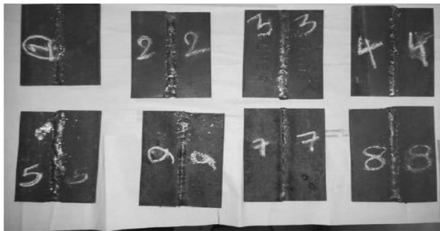
**Fig7: Specimen after welding operation**
