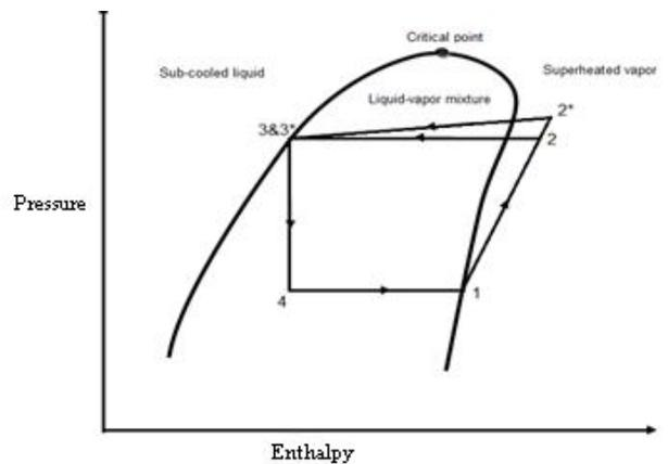
p-h diagram- VCRC with diffuser at outlet of compressor
