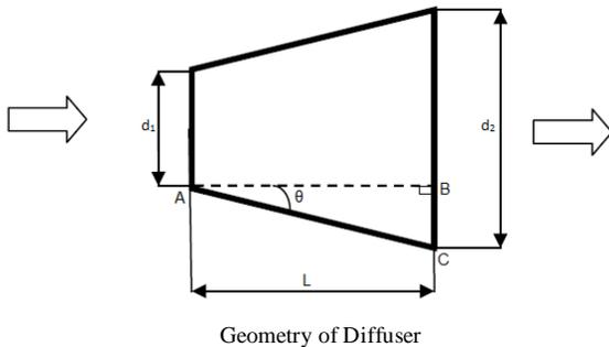
Diffuser's inlet and outlet diameters were designed. To design length of diffuser equation 1 is developed from figure1:
