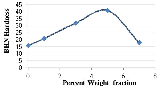
**Fig-1: Variation of Hardness with % weight fraction of reinforcement.**
