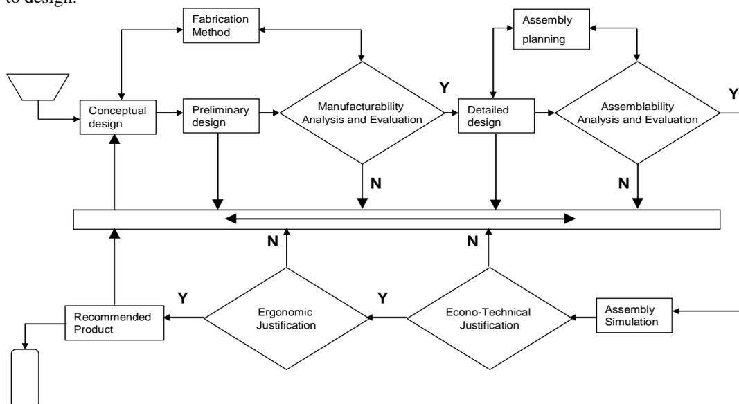
Fig. 1 – Integrated Assembly Oriented Design
