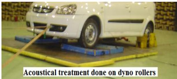
**Fig-4: Schematic of Indoor Pass-by noise Test set-up with Acoustical treatments**
